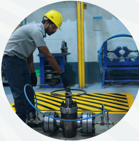
Gate Valve Testing
