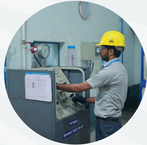
Gate Valve Testing
